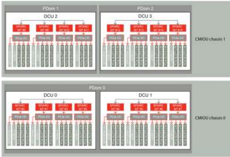
Figure 3. The SPARC M7-16 server can be flexibly configured with one, two, three, or four PDoms (three PDoms shown), each with two SPPs for active/passive failover.
