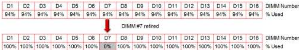
Figure 2. DIMM sparing provides for automatic failover of a single DIMM, with no interruption of service.
